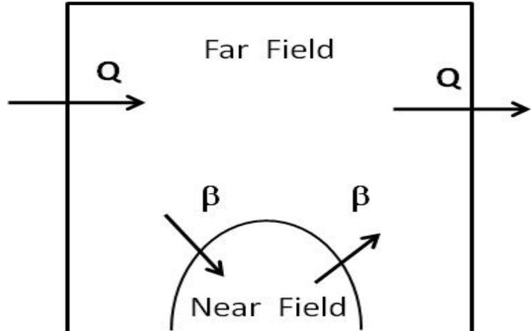
$$C_{NF}(t) = \frac{G}{Q} + \frac{G}{\beta} + G \left( \frac{\beta \cdot Q + \lambda_2 \cdot V_{NF}(\beta + Q)}{\beta \cdot Q \cdot V_{NF}(\lambda_1 - \lambda_2)} \right) \exp(\lambda_1 \cdot t) - G \left( \frac{\beta \cdot Q + \lambda_1 \cdot V_{NF}(\beta + Q)}{\beta \cdot Q \cdot V_{NF}(\lambda_1 - \lambda_2)} \right) \exp(\lambda_2 \cdot t)$$
